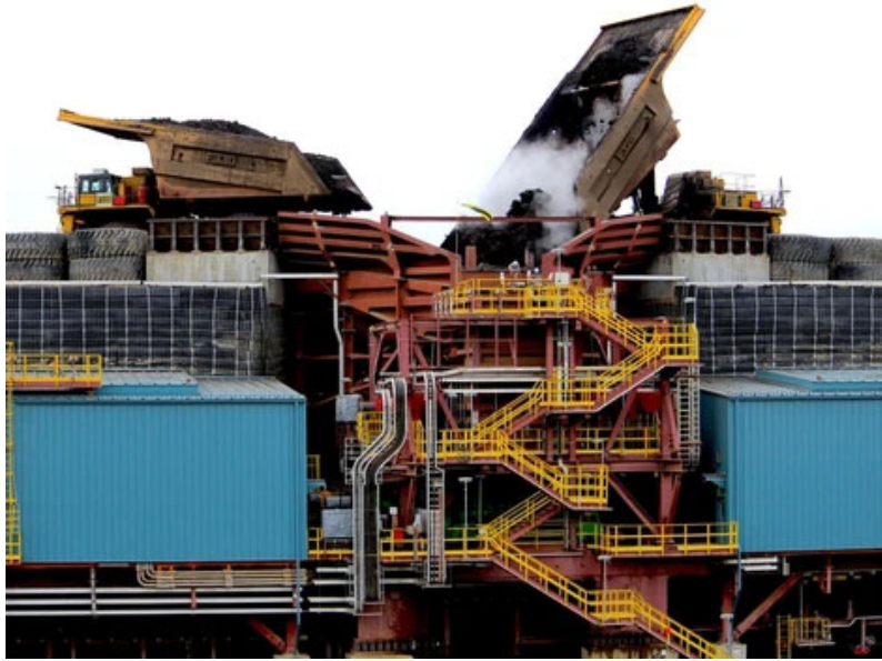
Heavy hauler trucks unload into a crusher at the Fort Hills oilsands project on Monday, September 10, 2018. Photo by Vincent McDermott / Postmedia
