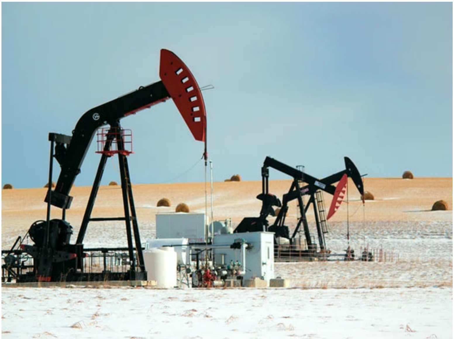
FILE PHOTO: Three operational pumpjacks adjacent to Sunset Ridge and Highway 22 battle through the winter chill on December 6, 2019. The horizontal wells, two operated by Ridgeback Resources and one by ORLEN Upstream, are producing oil from the Cardium formation. Patrick Gibson/Cochrane Times
