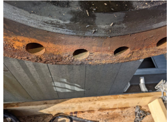
Sealing Surface Corrosion
