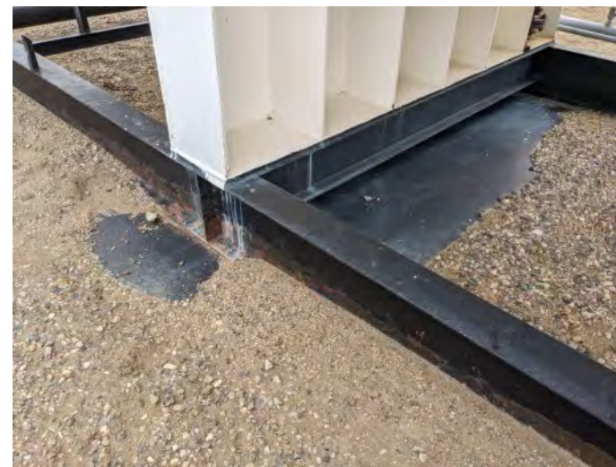
Saddle is welded to skid
