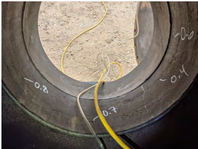
Manway nozzle corrosion
