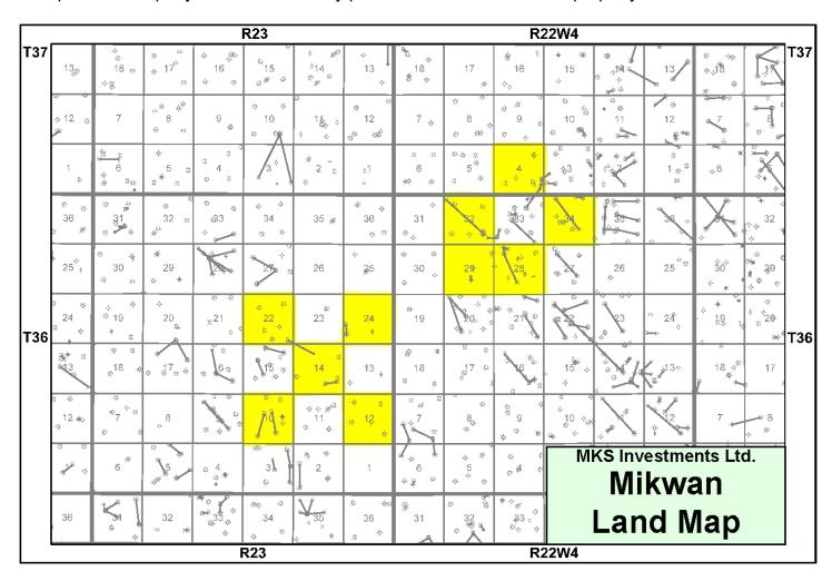
The Duvernay Formation at *Mikwan* is an upper Devonian marine shale reservoir. The Duvernay is found at a depth of approximately 2,000 metres and consists of approximately 10-15 metres of net pay using a 6% porosity cut-off.
