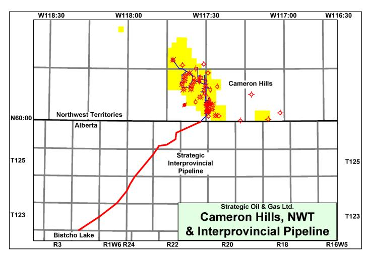
The Interprovincial Pipeline has been fully suspended, discontinued and properly cleaned and purged. Cathodic protection has been maintained on the pipeline. Information on the discontinuation and maintenance of the pipeline is available in the virtual data room for parties that execute a confidentiality agreement.
